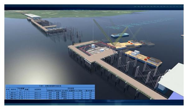
This multidiscipline model was also used for construction planning and simulation, helping the team evaluate in advance factors such as the proper position, angle, and route of the floating cranes used during construction. Navisworks simulation helped to arrange construction schedule, to make best use of human, machines and materials.
