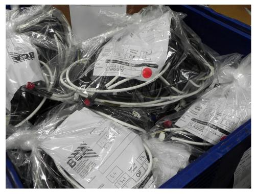
Figure 5: Ready for shipment, the harnesses are accompanied by delivery notes that carry data generated by  $E^3$  cable in order to provide complete traceability.
