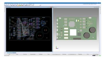
Fully functional and manufacturable electromechanical designs are created in a seamless ECAD-MCAD environment. Changes are highlighted interactively in both domains, minimizing design errors and shortening development time.
